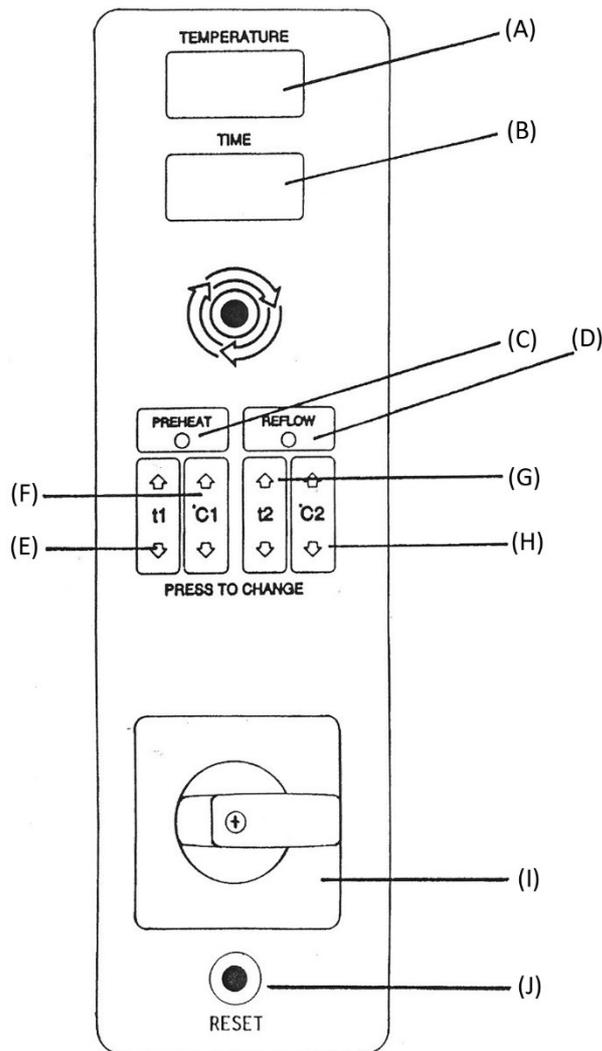
d. LED C is steady Red and LED D is blinking. The reflow process is running and you will see the quartz lamps are turned on. Both decimal points at the temperature display will be on and temperature is rising fast.
