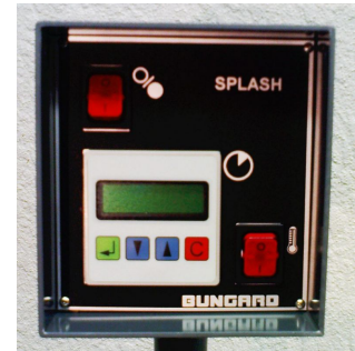
Control panel with new timer
