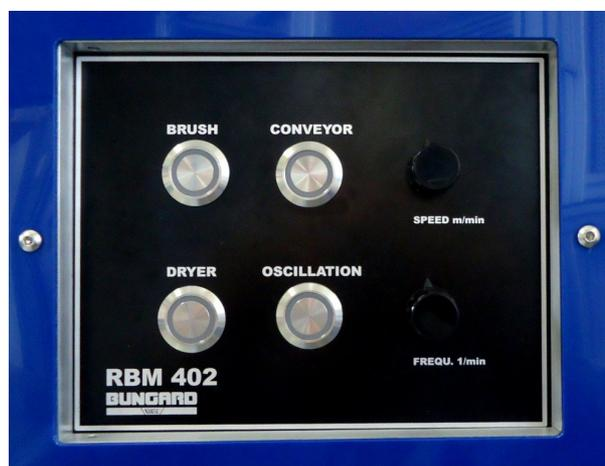
Switch on oscillation. Check that oscillation speed may be varied with potentiometer.
