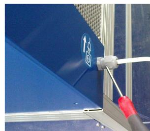
Block the brushing roller manually and loosen full floating axle clockwise (left-handed thread !) till you can pull it off.
