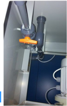
Ball Valve for the rinsing zone
