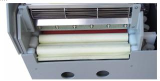
➤ The new cloth is fixed to the shaft without distortion with tape.
